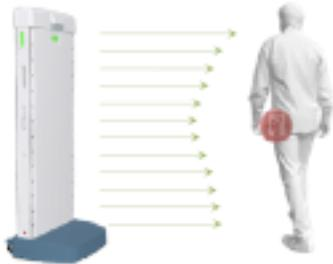
Low power signal is transmitted to reflect off the individual
